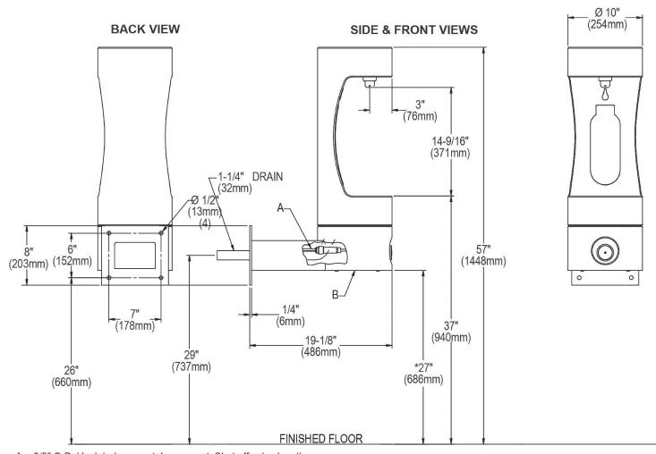
A = 3/8" O.D. Unplated copper tube connect. Shut off valve by others.  $B = Access panel(8" \times 10")$
